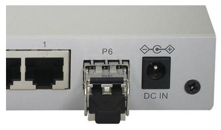
3. Until the SFP transceiver is seated securely in the slot, place the bail in lock position.
