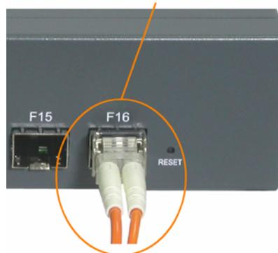
The following figure illustrates a connection example between two fiber ports:
