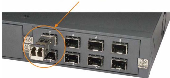
Insert SFP transceiver into a slot
