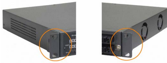
Install rack mounting brackets
