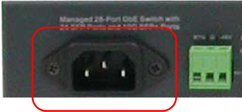
Figure 13: Inserting the AC power cord to AC socket to power on this switch
