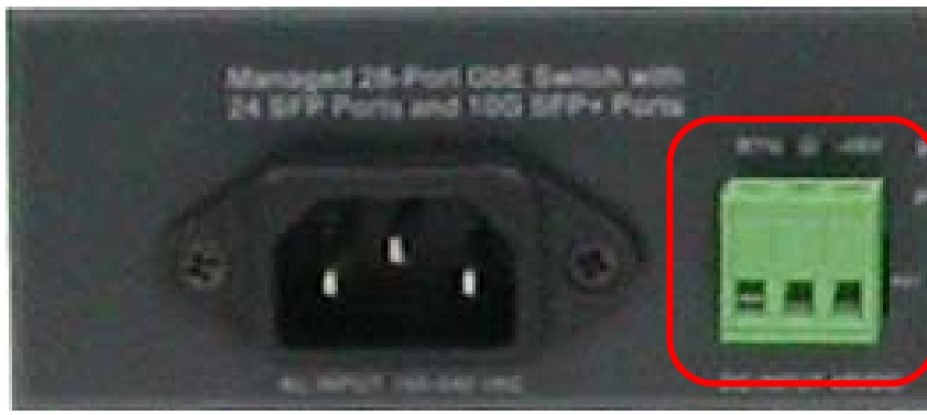
Figure 13: Inserting the DC Power cable to DC terminal block to power on this switch
